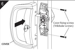
P Open door, and with the beak in the closed position and the key in the cylinder, place handle over lock. Rotate key if neccessary to engage cylinder into lock. Secure cover with cover fixing screws.
