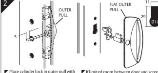
Maximum door thickness 45mm using a 5 pin cylinder in outer pull.
