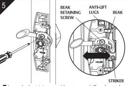
Loosen beak retaining screw (do not remove). Close door and engage beak with striker into desired position and retighten screws, do not overtighten. Check lock functions correctly.
